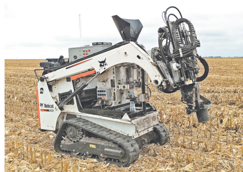
Figure 1. Robotic Sampler used on over 24,000 acres by Illini FS. Robotic sampling allows for improved accuracy and precision of soil sample collection, a must when collecting samples from dry, hard soils.
