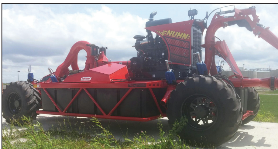
Above: Lagoon Crawler used to pull lime from water at a quicker rate, all with a remote control. With enhanced technology, the Crawler can drive itself out of a lagoon once empty.
